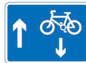
Figure 11-14 Diagram 960.2 (S9-4-7) Contraflow cycles with or without an advisory lane marked on the carriageway
